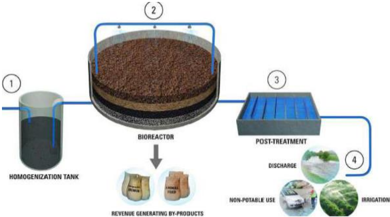
Aerobic Biofilter Without Sludge (ABWS)
