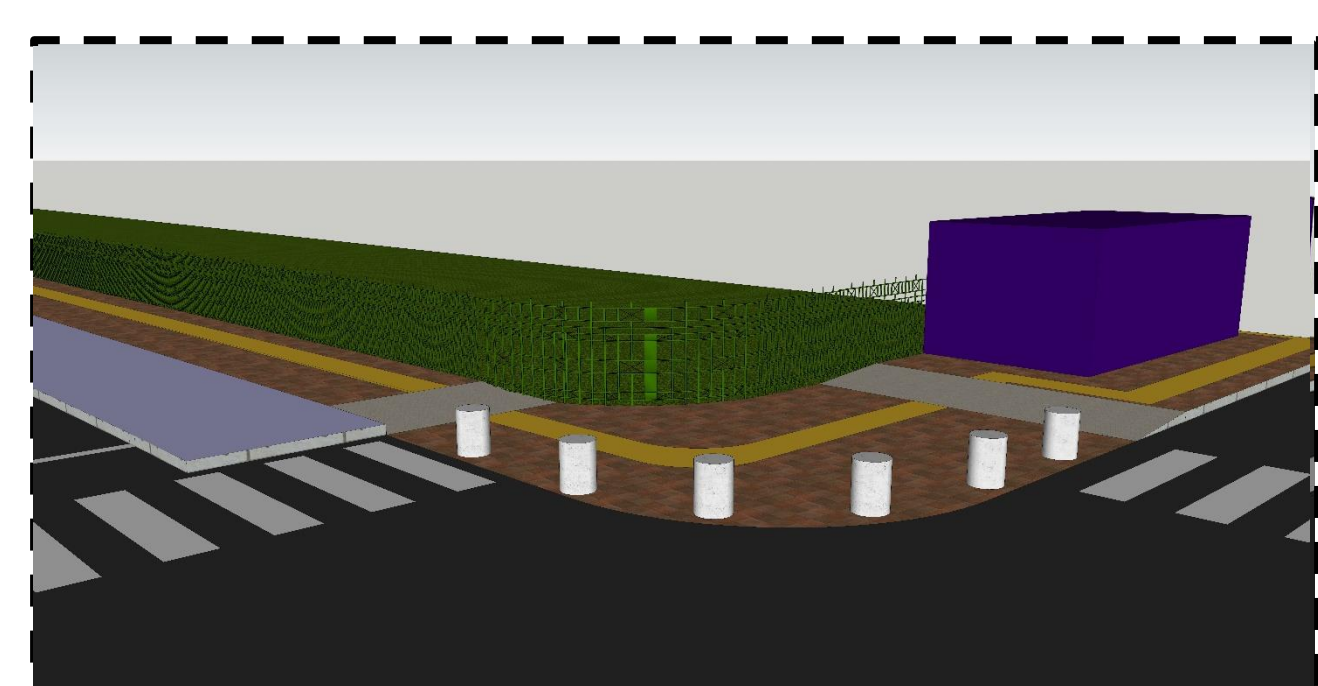
VIEW1: Ramps at Intersections Bollards at the turning to avoid traffic on footpath
